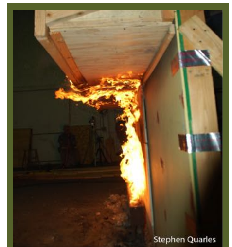
Lateral flame spread was reduced when a combustable soffit material ignited in this test of a soffited-eave with a combustable soffit material.
